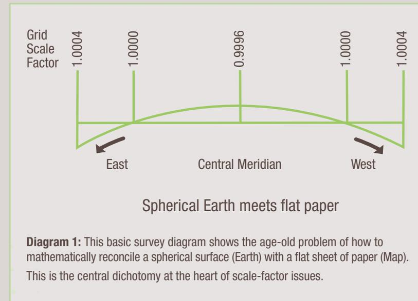
Depicting a **curved** surface (such as the earth) on a **flat** surface (such as on paper or in a digital representation of it), is a problem that surveyors solve using **map projections**. Map projections are not new and have been in common use for centuries. However, what *is* new is the increasingly widespread use of '**projected**' survey information: This has come about for **two** key reasons:
